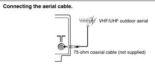
If you connect a VCR, connect the aerial output jack of your VCR and the aerial jack on the TV with the aerial cable. Then connect the output jacks of your VCR and the VIDEO-1 input jacks of the TV with the video cable and audio cables. For details, see the manual of your VCR.
