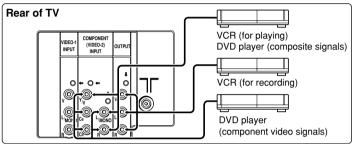
When connecting to COMPONENT (VIDEO-2) input, depending on the connection, choose the appropriate video input using the menu (see page 16).
